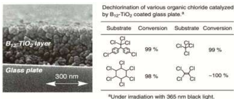
Figure 9. Immobilization of B 12 -TiO 2 hybrid catalyst onto glass plate.
